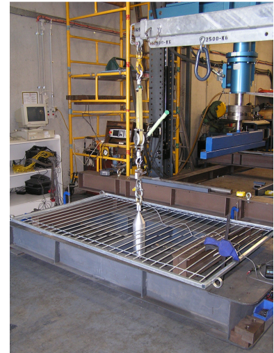
FIG.2. FENCE OPENING STRENGTH TEST
